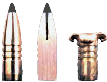
图1 SAKO公司.308 Win 480A POWERHEAD弹头形貌 Fig.1 Macroscopic feature of .308 Win 480A Powerhead
